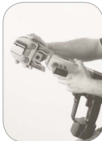
Place the jaws in the housing
